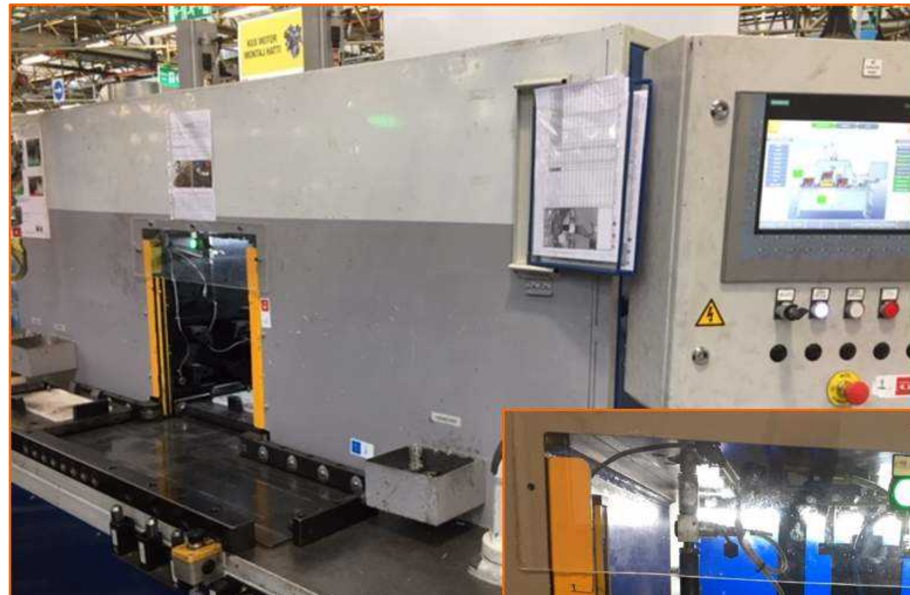
Pin Fastening To The Engine Block Servo Pres
